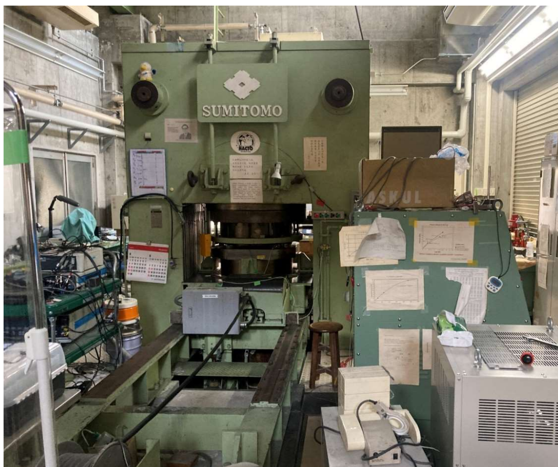
Fig.4 5000-ton KAWAI-Type Multi-Anvil Press
