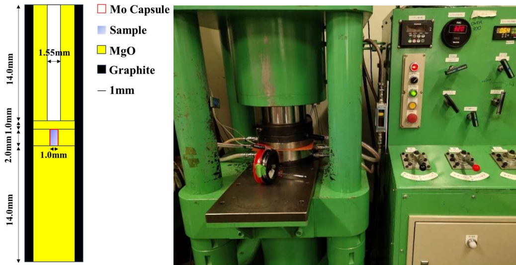
Fig.6 Schematic of Solidus Experiment Assembly and Piston-Cylinder Apparatus
